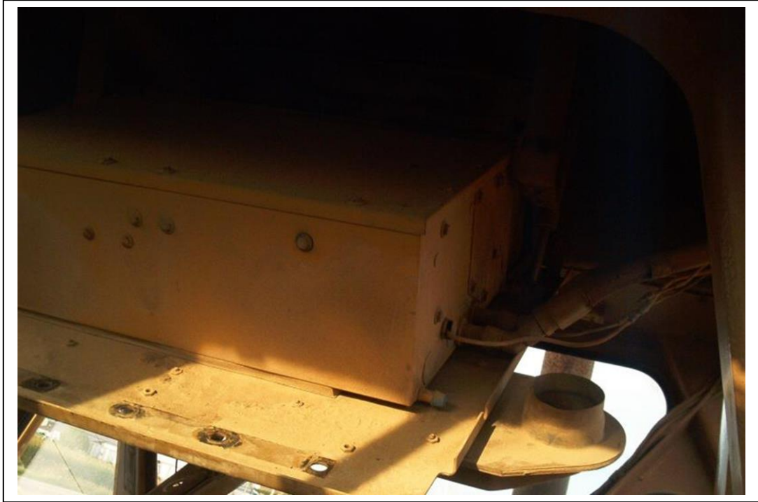
Ceiling panel and heater box lowered. Remove lid bolts and lid.
